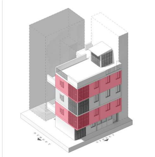
FIGURE 138 TYPICAL MODULE, STACKED FLATS ADJACENT TO EASTERN STAIRWELLS (DOWNHILL CORNERS), LEVELS 2 AND 4 SHOWN HIGHLIGHTED
