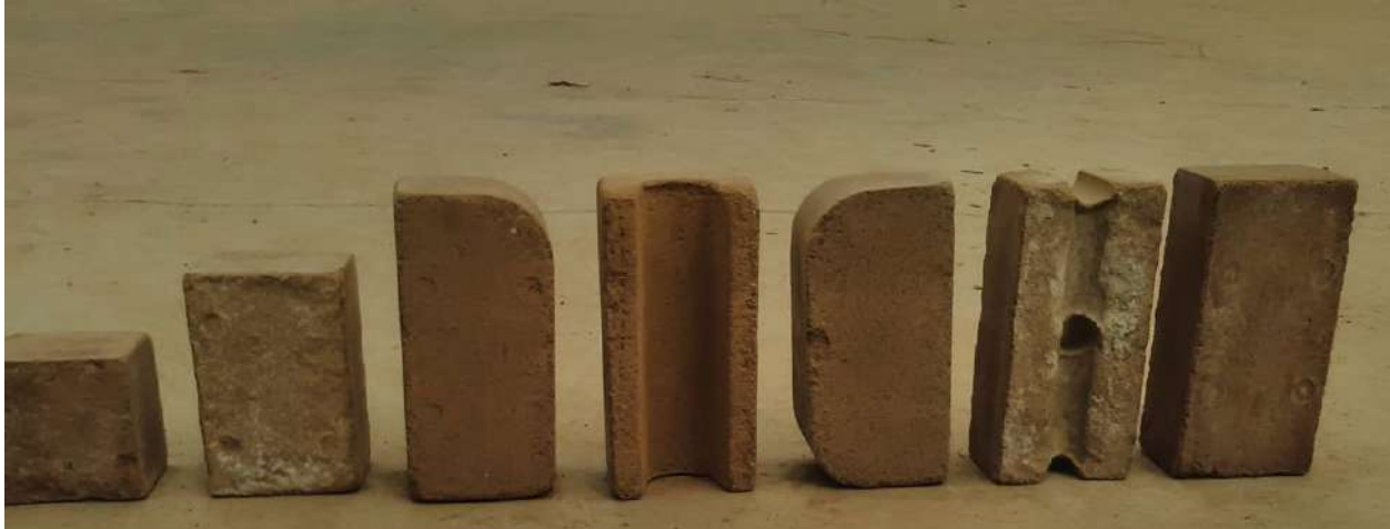
FIGURE 146 IMAGE OF VARIOUS SOIL BLOCKS USED IN ANGOLA
