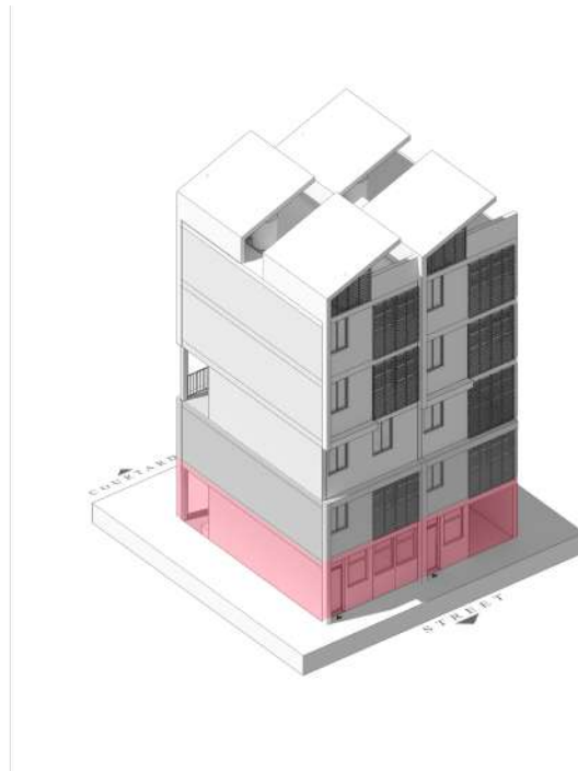
FIGURE 120 TYPICAL 5-UNIT MODULE FACING AN EAST/WEST STREET ON THE DOWNHILL SIDE (COURTYARD AT SAME LEVEL AS STREET) HIGHLIGHTING LOWER FLOORS OF LOWER TOWNHOUSE UNITS
