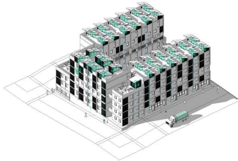
FIGURE 114 STORAGE TANKS FOR POTABLE WATER LOCATED ON ROOF
