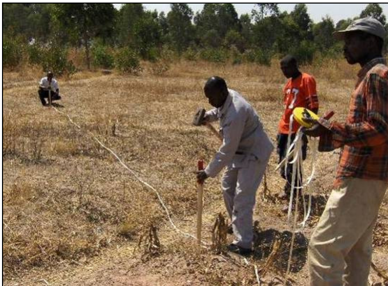
Fig. 5 Laying out new property boundaries
